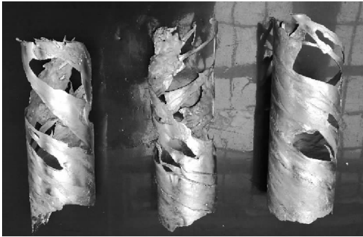
图 3 浇注温度为 690 ℃时,浆料在滚筒筒壁上形成的凝固壳 Fig.3 Solidified shell formed by slurry on the wall of barrel at the pouring temperature of 690 ℃
